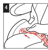
Push LATCH hook through the rear-facing belt path slot.
